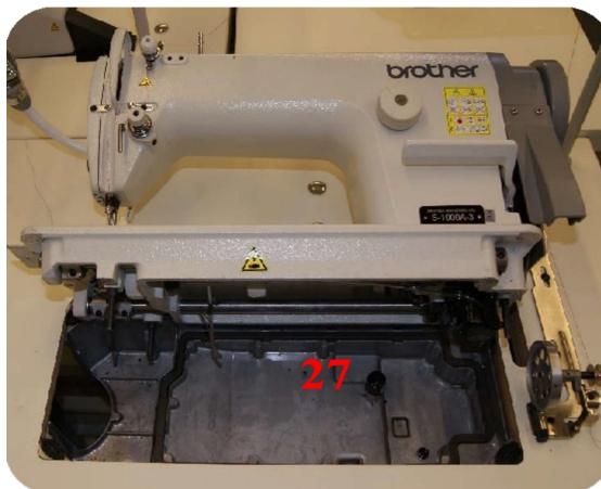
**27. Oil Reservoir:** Area underneath the machine that hold machine oil – machine must not be run if this reservoir is dry
