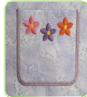
Faulty motifs or incorrect pocket position
