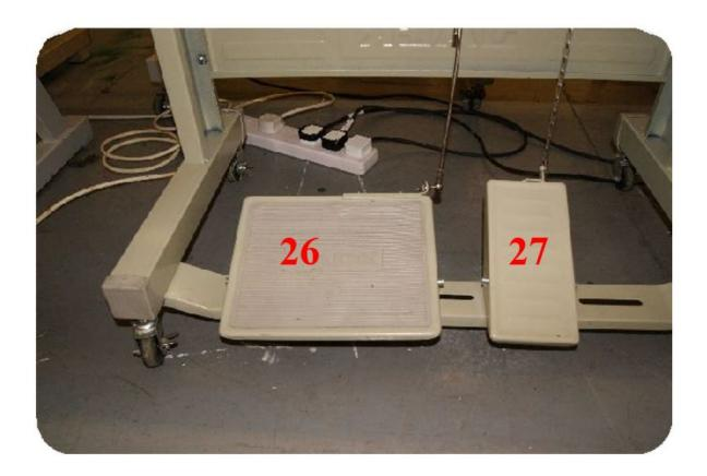
**26. Treadle:** Foot controls the sew, stops, starts, and controls speed of the machine
