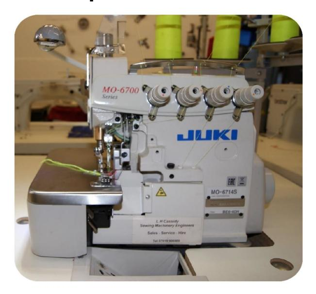
The overlocker above is a standard 4 thread twin needle made by JUKI, this machine sews a seam as it neatens. Four and five thread overlockers are the most used in the industry, because they create a strong flexible (stretchy) seam. However, there are a variety of different overlockers that use from one to five threads. They are used for various jobs as listed below:
