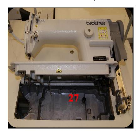
The oil pump is at the back of the pan; the oil is sucked up and distributed around the sewing machine, you will need to check the reservoir and remove thread waste, dust etc which will if left clog the oil and stop the lubrication process
