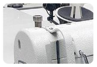
often preset. To make this adjustment, locate the pressure nub/screw. This is the presser spring regulator (usually on top of the machine, on left above/ behind the thread guide)
