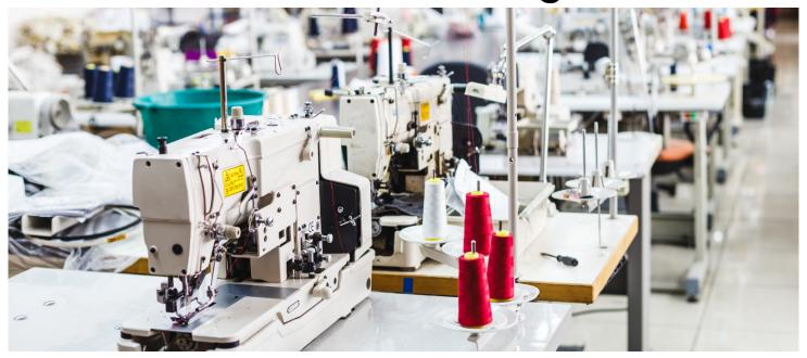
There are many different sewing machine models that cover various jobs, but most industrial models have a single function, for example, sewing straight seams, zigzag stitches, button attach, buttonholes etc. Attachments are often added to a machine to enable it to perform a certain function i.e., binding, ruffling, pleating.
